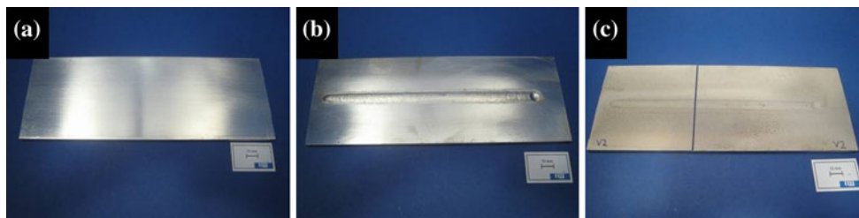
Fig. 6 Photographic images: a AZ31 raw material sheet; b a TIG welded seam of AZ31X on an AZ31 sheet; c coating of the welded seam prepared by SPS. The sample shown in c was cut in order to prepare the cross-section image shown in Fig. 7
